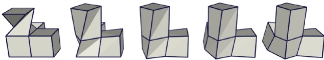
Figure 5: PQ perturbation without a closeness term applied to a highly un-planar mesh consisting of only a few quads.
