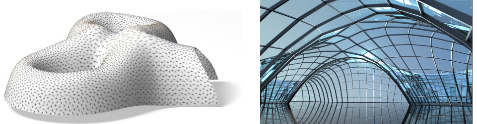
Figure 14: Planar quad remeshing of the surface of Figure 6. Left: Relative principal directions. Right: The result of optimization is a self-supporting PQ mesh, which guides a moment-free steel/glass construction (interior view, see also Fig. 1).
