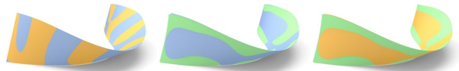
Figure 24: Approximation by ruled surfaces of different kinds: A reference surface (blue) which is an unmodified part of the Cagliari museum project by Zaha Hadid architects is approximated by Flöry et al. [33] with a conoidal ruled surface (green) and with a general ruled surface (orange). We show these surfaces superimposed onto each other in order to visualize approximation quality.
