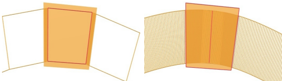
Figure 14: Discrete developable surfaces and their smooth counterparts. A strip of planar quadrilaterals is called a discrete developable, because firstly it can be unfolded into the plane, and secondly refinement of such a strip where quads retain their height but their width goes to zero produces, in the limit, a smooth developable surface. Under this limiting procedure, the planes which contain individual quads converge to the tangent planes of the smooth limit surface.
