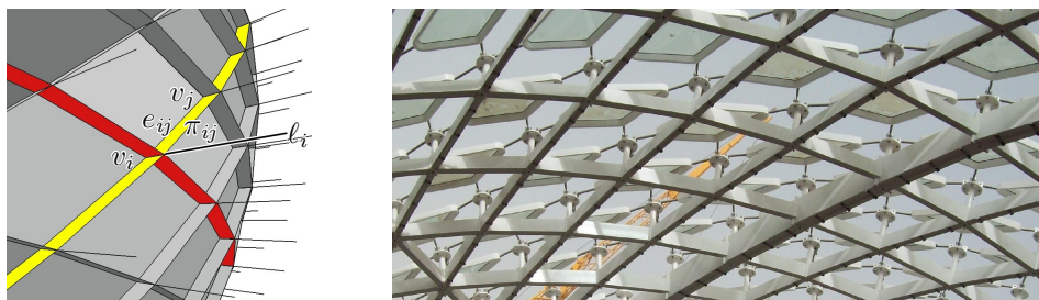
Figure 4. Torsion-free support structure. For each edge ij and vertex i of a quadrilateral mesh, we have a plane \pi_{ij} and a line l_i such that e_{ij}, l_i, l_j are contained in \pi_{ij} (at left, image courtesy Evolute). This support structure guides members and nodes in the outer hull of the Yas Marina hotel in Abu Dhabi, so that members have a nice intersection in each node (at right, image courtesy Waagner-Biro Stahlbau).
