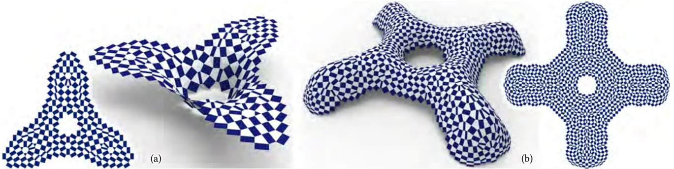
Fig. 21. 2D checkerboard patterns lifted to 3D while still retaining that the black rectangles of the same type have the same aspect ratio.
