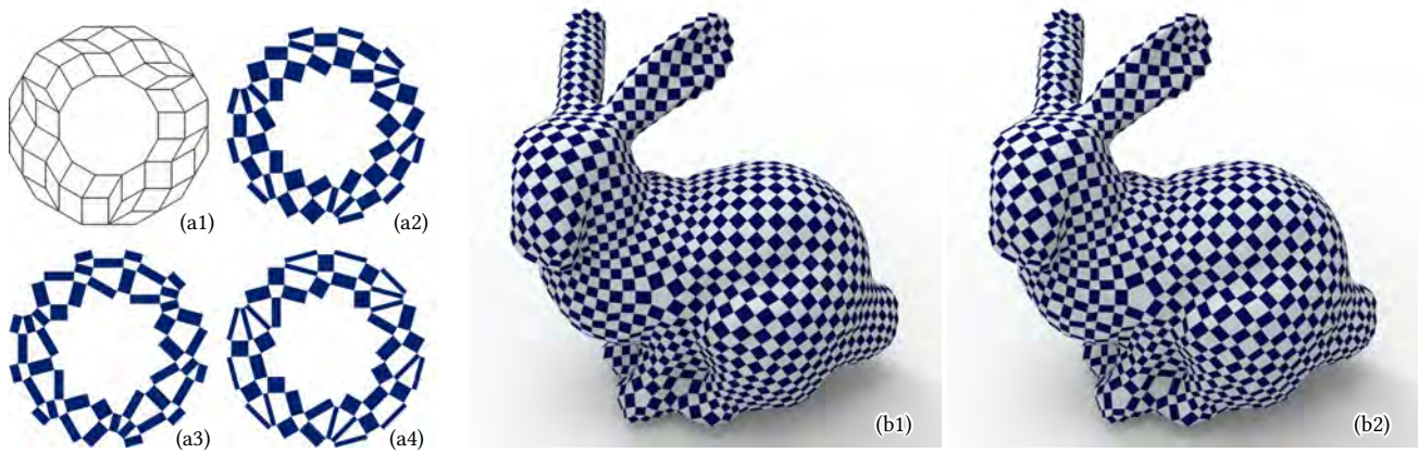
Fig. 4. (a1) The control mesh for the Tokyo 2020 Olympics Games logo design. (a2) to (a4): checkerboard patterns generated from the same control mesh but with different \lambda for the interpolation of the two diagonal meshes. (a2) is the logo ( \lambda = 0.5 ). (b1) and (b2): Two 3D checkerboard patterns generated from the same control mesh but with different \lambda .
