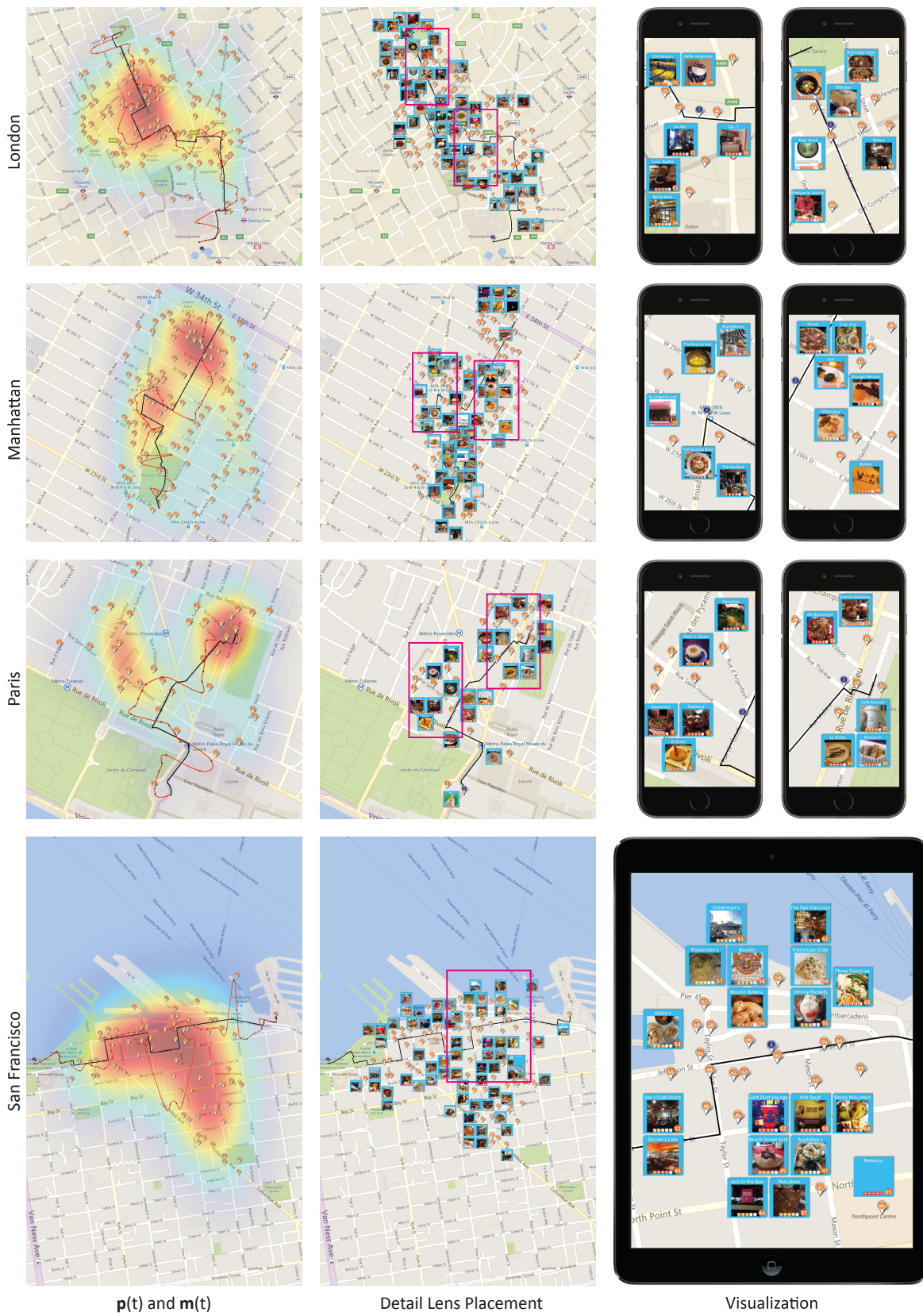
Fig. 16: Results of our framework. (left) Overview of the example areas with the queried set of POIs P and the computed paths p(t) (black) and m(t) (dark orange). The sum of the mixture of POI Gaussians, indicating the POI distribution, is outlined by a heat-map. (middle) The computed positions of the detail lenses. Note that the overlaps do not occur in the final visualization due to placement in different time spans. (right) Example views of the final visualization for different mobile devices (iPhone 6 Plus and iPad Air 2).
