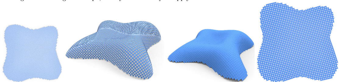
Figure 13: For a given surface in space, we can design a cut pattern in the plane deploying continuously to that surface (figures at left). The expansion can also go the other way — on a given surface we design a cut pattern that causes deployment to a planar domain (figures at right).
