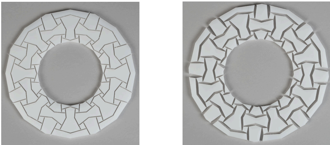
Figure 6: A 2D bistable auxetic metamaterial based on an underlying quad pattern.
