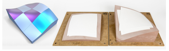
Fig. 18. Paneling free forms. The rendering at left shows a covering of the design surface by panels categorized according to Gaussian curvature K . We fabricated them by minimally altering the shape via optimization so that we need only two molds (at right): a spherical mold corresponding to 2 panels exhibiting K > 0 ; a mold with constant negative Gaussian curvature corresponding to 3 panels; and a virtual flat “mold” corresponding to 4 developable panels. See Fig. 19 for the final result.
