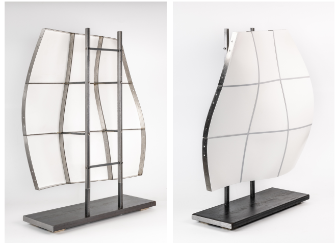
Fig. 19. Paneling free forms with an isometrically deforming material. This is an actual model built with high impact polystyrene panels. For the design surface and a photo of the molds see Fig. 18.
