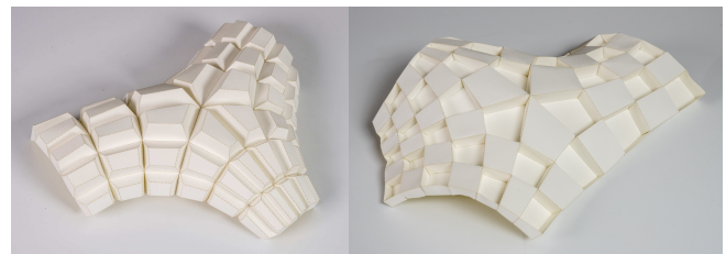
Fig. 23. Box kirigami structures are here made from paper that has been cut and perforated by a laser. We show a type B kirigami (left) and a type C kirigami (right) which is particularly rigid.
