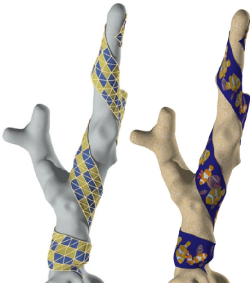
Fig. 9 Fair polygon network used for texture mapping. The mean size of features of the coral branch implies that the network is just dense enough to avoid being stuck in an insignificant local minimum. Experimental evidence supports this. The colored band itself lies on the given surface.
