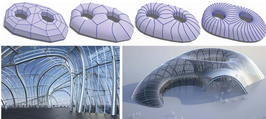
An example of construction-aware geometric design. Combining subdivision and optimization (top) provides a direct approach to modeling freeform surfaces which are composed of single-curved strips. A result of this technique is shown in the two views of a research case study (bottom).
