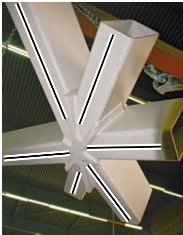
Figure 1: Node with Torsion . Manufacturing a vertex where symmetry planes of incoming beams do not intersect properly is demanding, especially the central part (image courtesy Waagner-Biro Stahlbau).
