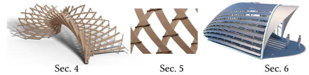
Fig. 4. Overview of applications. Gridshells formed by two or three families of rectifying strips are presented in Sec. 4 along with physical models. The difficult topic of gridshells with torsion-free nodes, where transversal strips meet at straight line segments, is addressed in Sec. 5. In Sec. 6 we design shading systems via a single family of rectifying strips.
